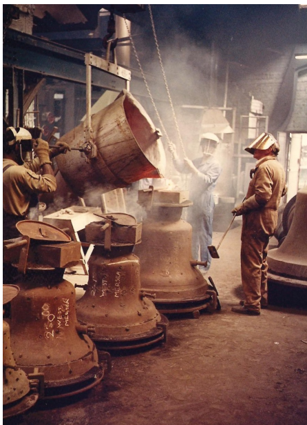
Taylor's cast their bells with the moulds buried in pits below ground level. The bells being cast in these photos are not especially large, but they are standing on the floor of the foundry. It does get rather exciting if one of the moulds fails! They have had more than one fire as a result.
